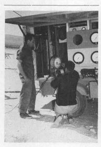
THE CALIBRATION TRAILER is the scene of operations here as Sgt. Ron Meinert, left, and Robert Thompson work on a pressure standard. Instruments were continually adjusted and tested to keep them in top condition.
